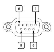
Figure 3.1 Serial DB9 Console Port
