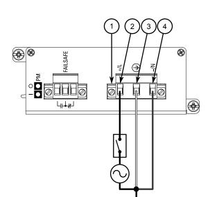
1. Connect the power supply terminal block to the device.
