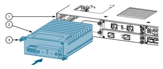
Figure 4.6 Installing a Power Module
