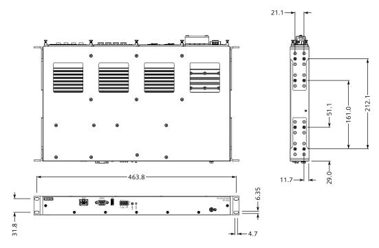
Figure 5.2 Rack Mount Dimensions
