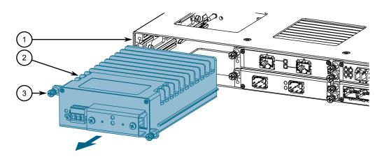
Figure 4.5 Removing a Power Supply
