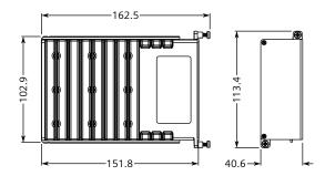
Figure 5.5 Power Module Dimensions
