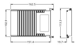
Figure 5.4 Line Module Dimensions
